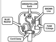
As the colours of the wires in the mains lead of this appliance may not correspond with the colour markings identifying the terminals in your plug, proceed as follows. The blue wire must be connected to the terminal marked with an N or coloured
